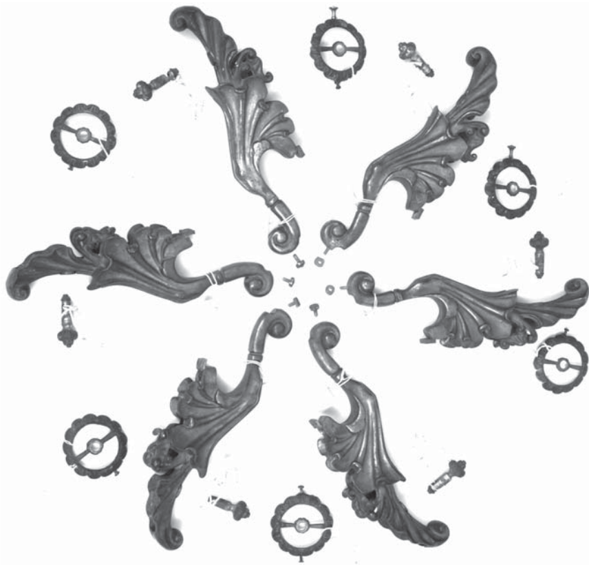
Disassembled and labeled rear parlor gaselier depicting the cast arms, shade holders and gas valves during the conservation treatment. Photograph by conservator Julie Baker.
